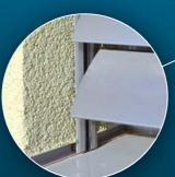
Hidden guiding rail - creates a uniform and clean appearance of a building when the hidden rails are inserted in the facade **Upper profile** (aluminium or zinc coated steel) - turned down - this position prevents sticking of dirt in the upper profile, easy access to control the blind (when servicing the blinds)
